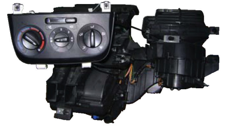
● Air Conditioning System / Klima Sistemi FIAT FIORINO - PEUGEOT BIPPER - CITROËN NEMO
